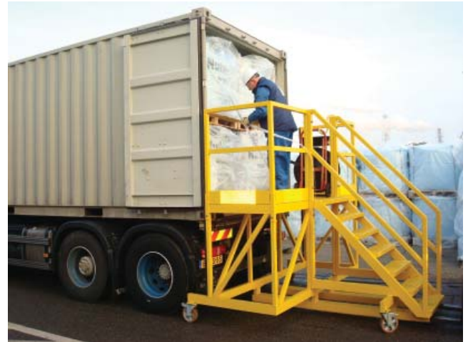
New fall protection while loading containers
