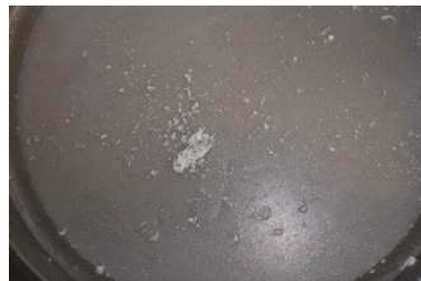
Generic epoxiconazole tank mixture through a 300µm sieve
