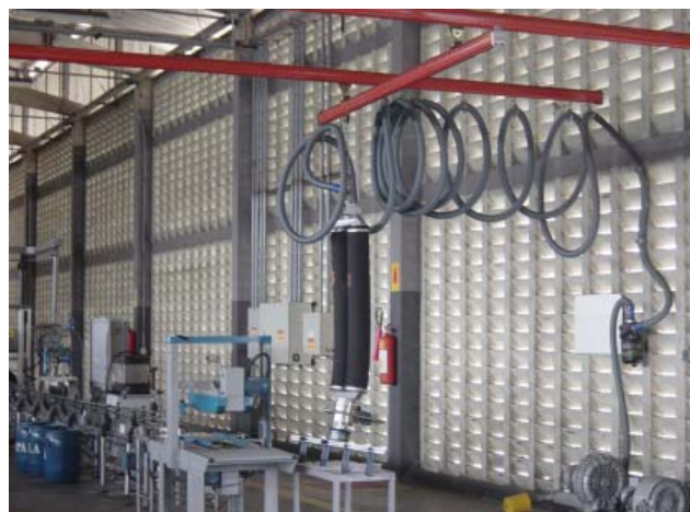
Vacuum lifting aid for handling drums onto pallets
