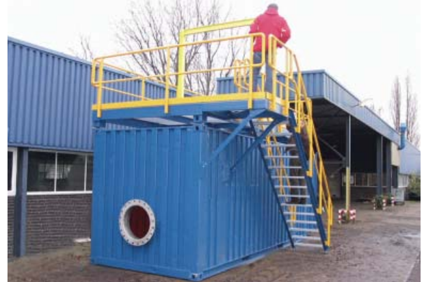
Training rig for confined space rescue
