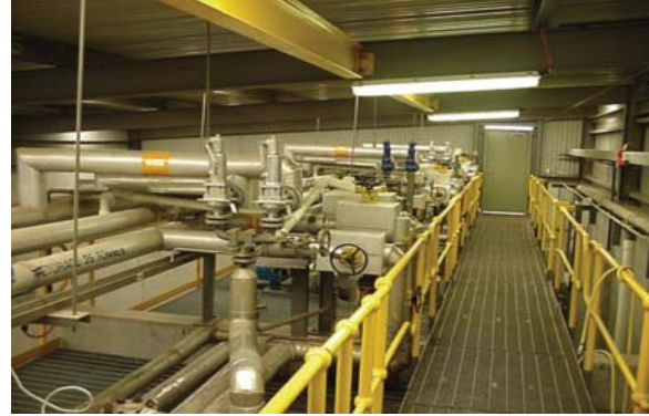
Liquid chlorine being evaporated for export to Tiwest as gaseous chlorine
